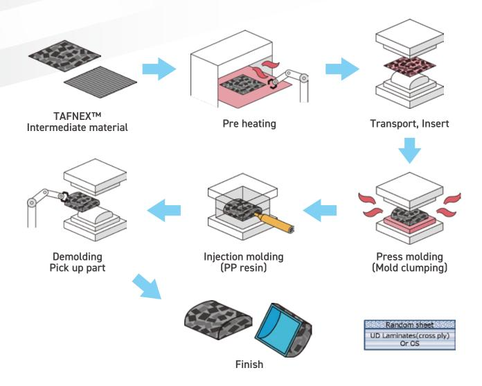
Over molding process: Heat press + Injection molding
